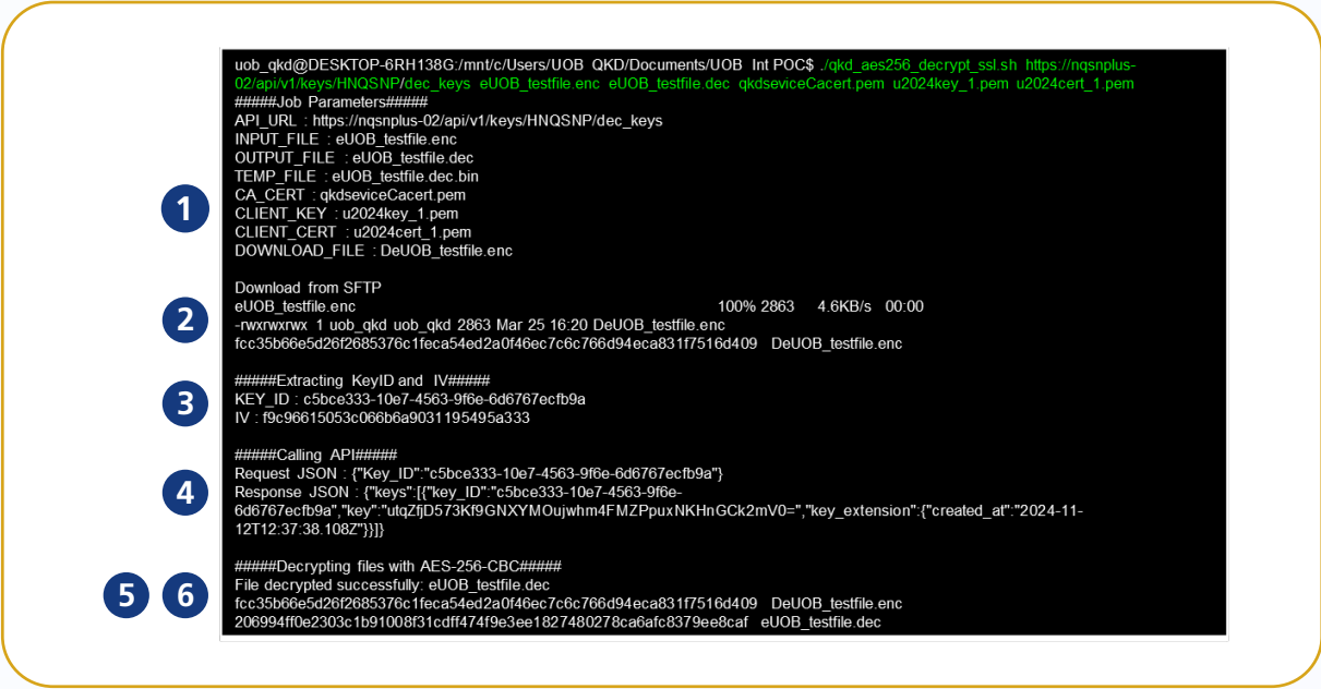
Figure E-4: Decryption process for use of QKD with AES-256 for an automated file transfer leveraging SFTP
